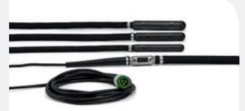
ELECTRIC-POWERED HUSQVARNA VIBRASTAR 42 V–3–200 Hz, Ø 40–60 mm, hose length 5 m, 8.4–15 kg.
