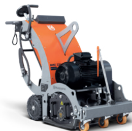
ELECTRIC-POWERED HUSQVARNA BMC 335 16 kW, 400V/32-63 A, 3-phase, 335 mm working width, 430 kg.
