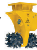
HYDRAULIC-POWERED HUSQVARNA DXR 305 27 kW, 1960 kg, reach 5.2/4.9 m up/forward incl. tool.
