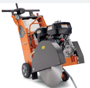
PETROL-POWERED HUSQVARNA FS 400 LV Diamond blade max 450/500 mm, cutting depth 162 / 189 mm, 99 kg, 8.7 kW*.
