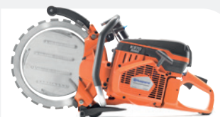
PETROL-POWERED HUSQVARNA K 970 RING 94 cc, 4.8 kW, 13.8 kg, blade size 370 mm, cutting depth 270 mm.
