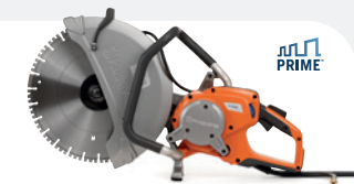
ELECTRIC-POWERED HUSQVARNA K 7000 230/400 V, 5.5 kW (3-phase)/3 kW (1-phase), 9.8 kg, blade size 400 mm, cutting depth 155 mm.
