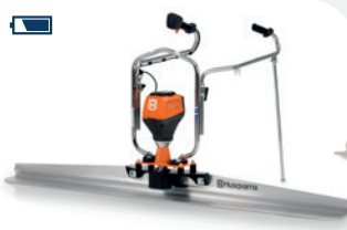
BATTERY-POWERED HUSQVARNA BV 30i Output power 1.4 kW, output power 0.8 kW, weight 11.5 kg, BLi 36 V battery system.
