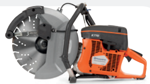
PETROL-POWERED HUSQVARNA K 770 SMARTGUARD 74 cc, 3.7 kW, 10.8/11.1 kg, blade size 300/350 mm, cutting depth 100/125 mm.
