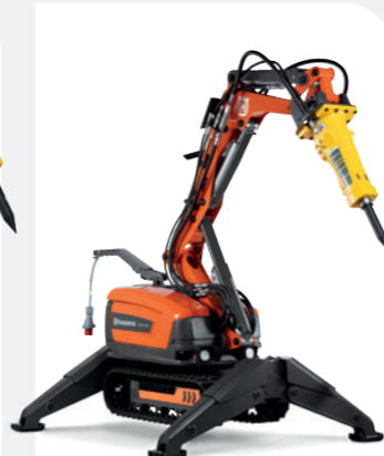
HYDRAULIC-POWERED HUSQVARNA DXR 275 24 kW, 1750 kg, reach 4.8/4.5 m up/forward incl. tool.
