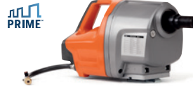
ELECTRIC-POWERED HUSQVARNA DM 700 6000/3000 W, 3-phase/1-phase, recommended drill diameter 80–600 mm, 14 kg.
