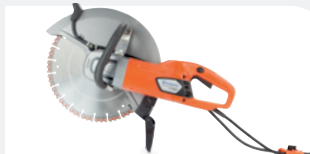
ELECTRIC-POWERED HUSQVARNA K 4000 230/120/110 V, 2700/1800/2200 W, 8.5 kg (incl. Vac attachment 1 kg), blade size 350 mm, max. cutting depth 125 mm.
