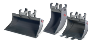
HUSQVARNA BUCKETS Available in three sizes. For DXR DXR 140/145: Standard 52 cm/55 liters. Wide 77 cm/60 liters. Narrow 30 cm/40 liters. All other DXRs: Standard 52 cm/85 liters. Wide 77 cm/105 liters. Narrow 30 cm/40 liters.
