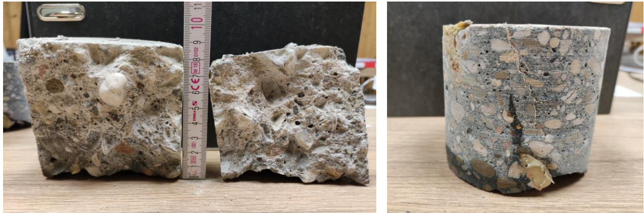
Core samples from slab treated with Krystaline 1 demonstrating penetration and crack self-healing six weeks after application
